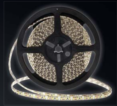
968 (3000K) 969 (6000K) 12V, 3528 120LED/m, 9,6W/m 5m roll klasa ochronności / protection class - IP20
