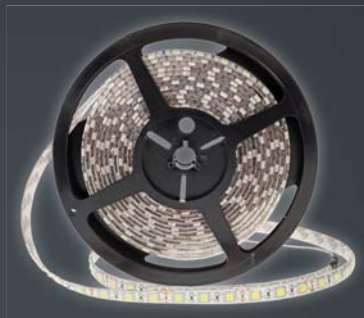
970 (3000K) 978 (6000K) 12V, 5050 60LED/m, 14,4W/m 5m roll klasa ochronności / protection class - IP20
