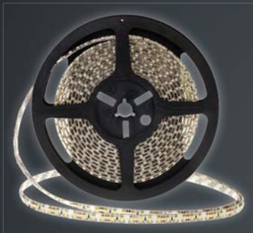
974 (3000K) 975 (6000K) 12V, 3528 120LED/m, 9,6W/m 5m roll klasa ochronności / protection class - IP65
