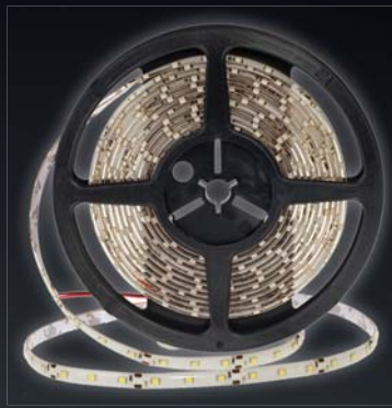
972 (3000K) 973 (6000K) 12V, 3528 60LED/m, 4,8W/m 5m roll klasa ochronności / protection class - IP65
